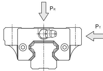
For the case of mono rail, the moment effect should be considered. The equation is:
