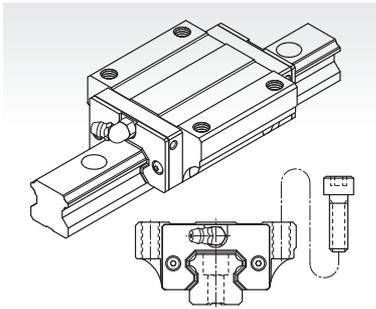
Installed from top side of carriage with the thread length longer than MSA-E type.
