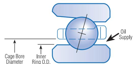
Fig. 17. Lubrication window for B-type bearings.
