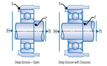
**Table 49.** Shaft and housing shoulder diameter abutment dimensions for deep groove spindle & turbine (metric) bearings.
