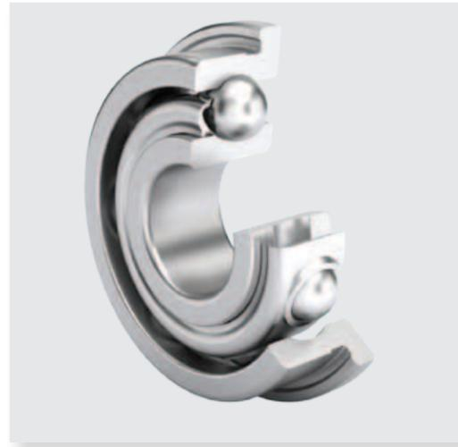
Flanged bearings provide solid mounting for good axial control and eliminate the need for housing shoulders or shoulder rings. Housings can be through-bored to reduce manufacturing costs and simplify assembly. When flanged bearings are used, the housing mounting surfaces must be accurately machined to properly position and support the bearings.
